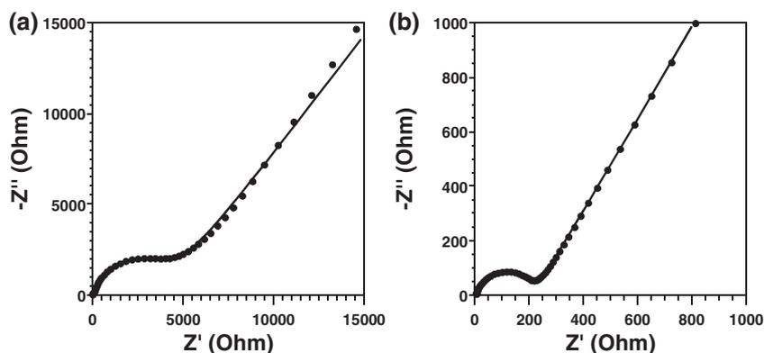
**Figure 5.** Nyquist plots of graphite anodes in EC:PC electrolytes obtained in EIS test in a) K-ion and b) Li-ion batteries after three activation cycles. The solid lines are the fitting curves by using the equivalent circuits which are shown in Figure S9 (Supporting Information).
