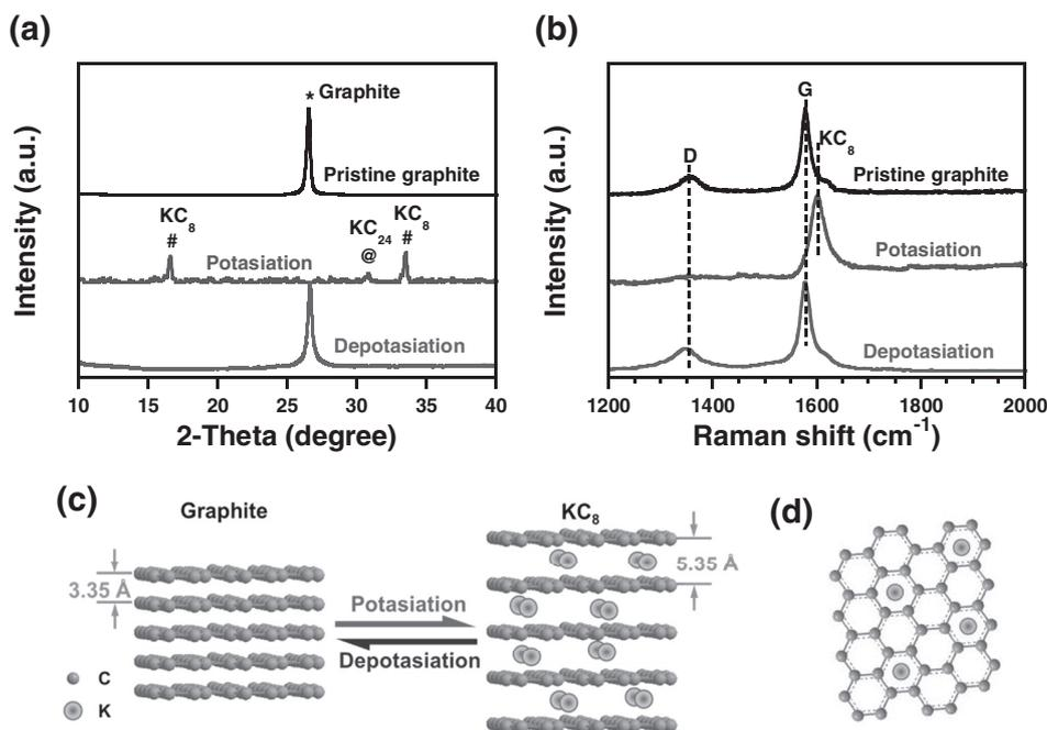
**Figure 2.** a) XRD pattern and b) Raman spectra of fresh graphite anodes and at potasiation and depotatiation states. c) Schematic illustration of potasiation/depotatiation processes of graphite, which shows the interlayer distance expanded from 3.35 to 5.35 Å upon the intercalation of K, and d) schematic diagram of in-plane pattern for KC<sub>8</sub>.
