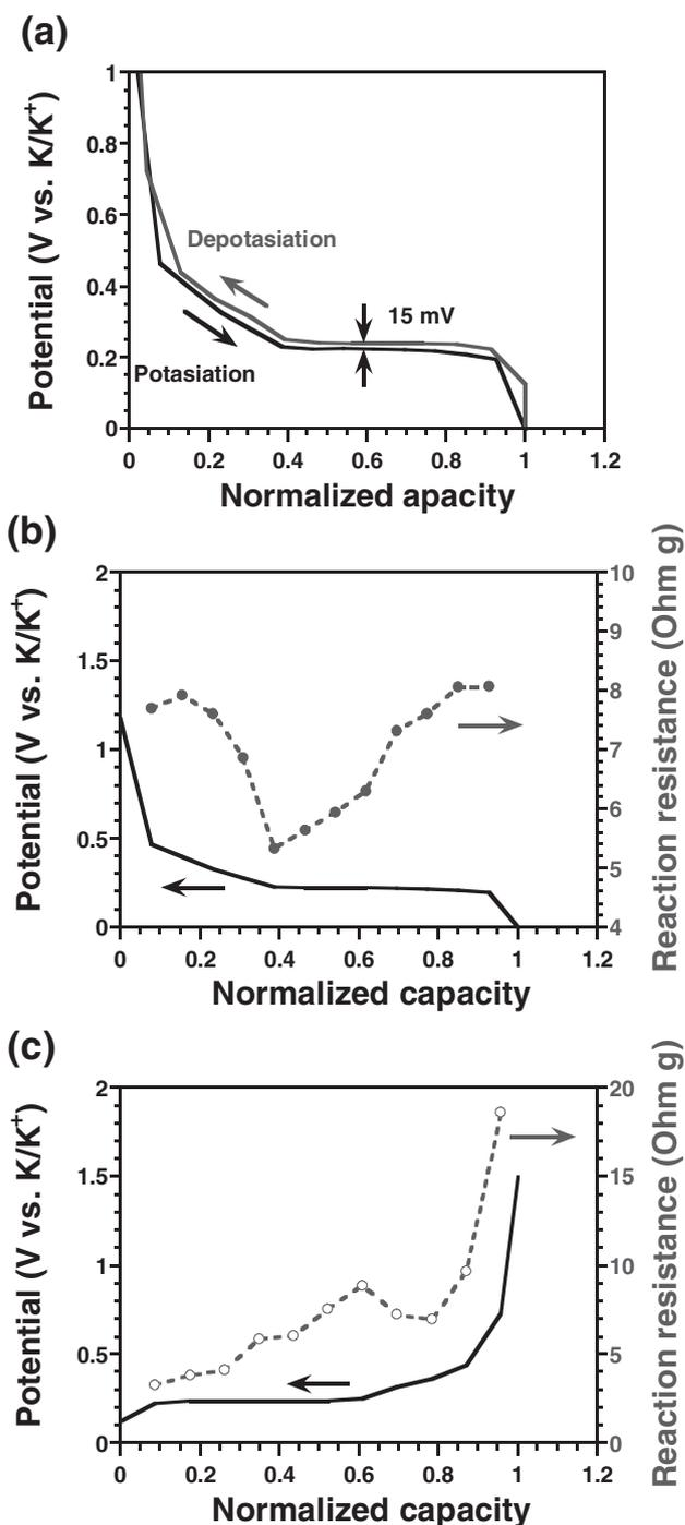
**Figure 4.** a) Quasi-thermodynamically equilibrium potential profiles and reaction resistance during b) potasiation and c) depotasiation processes of graphite in K-ion batteries in EC:PC electrolyte. For comparison, the capacity was normalized to the maximum potasiation/depotasiation capacity values.
