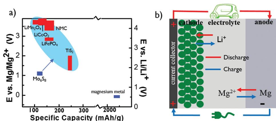
**Figure 1.** Schematic of a) the potential and capacity of a magnesium-ion battery's cathode (Mo<sub>6</sub>S<sub>8</sub>), anode (magnesium metal), and some lithium-ion battery cathodes that could possibly be used in the mixed-ion battery; b) the operating mechanism of the mixed-ion battery.
