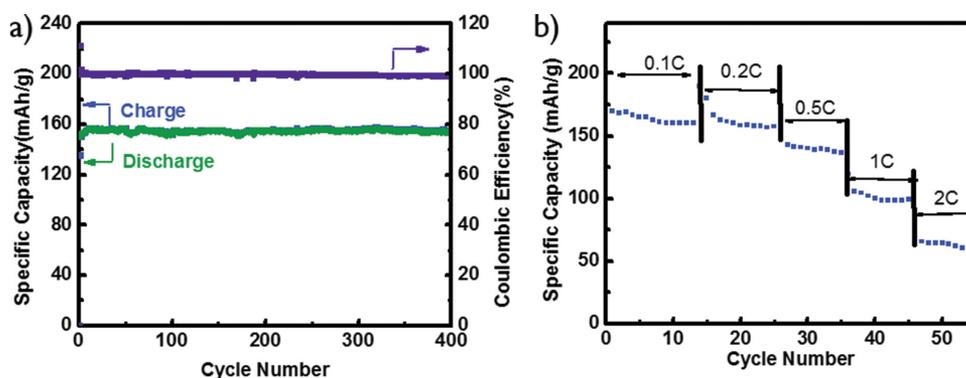
Figure 3. a) Cycling stability at C/3 and b) rate capability of a  $\text{TiS}_2|\text{Li}^+, \text{Mg}^{2+}|\text{Mg}$  battery.
