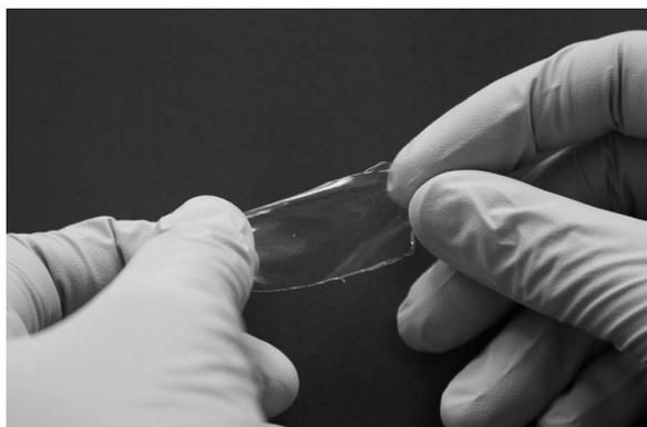
**Figure 1.** Electrolyte membrane constructed from the diblock copolymer PEO-*b*-(PMMA-*ran*-PMAALi) and the LiBOB salt (picture taken shortly after removal from an argon glove box).
