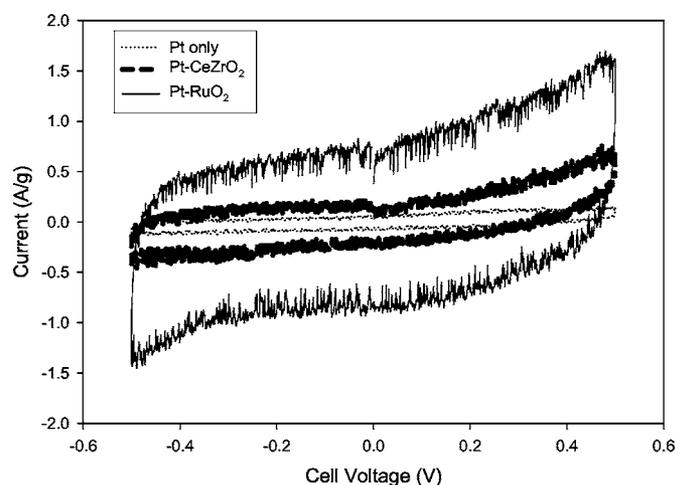
**Figure 5.** CV of the PEMFCs with and without energy storage element addition in  $\text{N}_2$  environment at a scan rate of 5 mV/s. Pt loading: 0.3 mg/cm<sup>2</sup>, CeZr loading: 0.6 mg/cm<sup>2</sup>,  $\text{RuO}_2 \cdot x\text{H}_2\text{O}$  loading: 0.6 mg/cm<sup>2</sup>.
