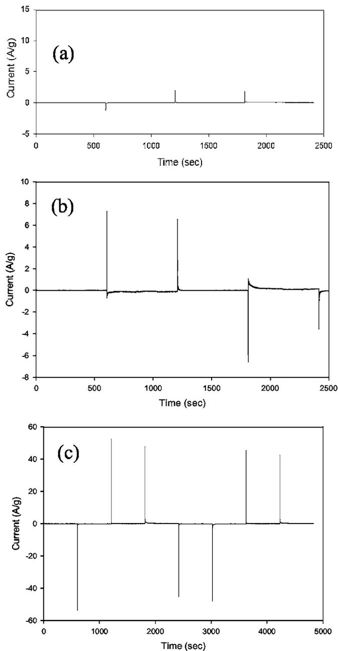
**Figure 7.** Pulse-loading performance of the PEMFCs with and without energy storage element addition measured using the pulse voltammetry program in Fig. 3 under the humidified nitrogen atmosphere, (a) Pt loading:  $0.3 \text{ mg/cm}^2$ , (b) Pt ( $0.3 \text{ mg/cm}^2$ )- $\text{CeZrO}_2$  ( $0.6 \text{ mg/cm}^2$ ), and (c) Pt ( $0.3 \text{ mg/cm}^2$ )- $\text{RuO}_2 \cdot 0.5\text{H}_2\text{O}$  ( $0.6 \text{ mg/cm}^2$ ).
