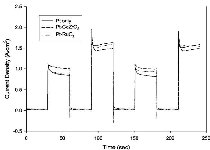
**Figure 8.** Pulse-loading performance of the PEMFCs with energy storage elements addition measured by the potential square-wave voltammetry program in Fig. 3. Pt loading: 0.3 mg/cm<sup>2</sup>, CeZrO<sub>2</sub> loading: 0.6 mg/cm<sup>2</sup>, RuO<sub>2</sub>·0.5H<sub>2</sub>O loading: 0.6 mg/cm<sup>2</sup>.
