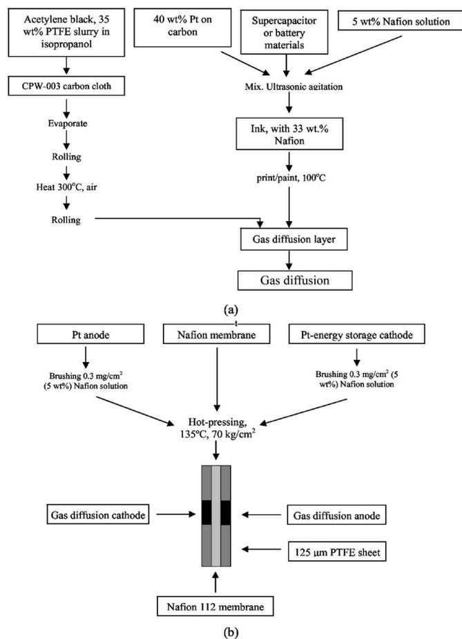
**Figure 1.** Preparation of (a) gas diffusion electrode and (b) MEA used for the internal PEMFC/energy storage hybrid power system.
