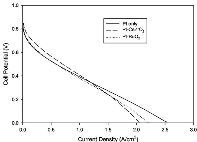
**Figure 6.** Steady-state performance of the PEMFCs with and without energy storage element addition. Pt loading:  $0.3 \text{ mg/cm}^2$ ,  $\text{RuO}_2 \cdot 0.5\text{H}_2\text{O}$  loading:  $0.6 \text{ mg/cm}^2$ ;  $\text{CeZrO}_2$  loading:  $0.6 \text{ mg/cm}^2$ .
