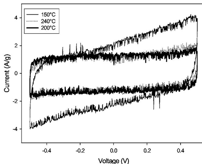
**Figure 4.** CV of the PEMFC with annealed  $\text{RuO}_2 \cdot x\text{H}_2\text{O}$  addition at 10 mV/s in  $\text{N}_2$  environment. Pt loading: 0.6 mg/cm<sup>2</sup>,  $\text{RuO}_2 \cdot x\text{H}_2\text{O}$  loading: 1.1 mg/cm<sup>2</sup>.
