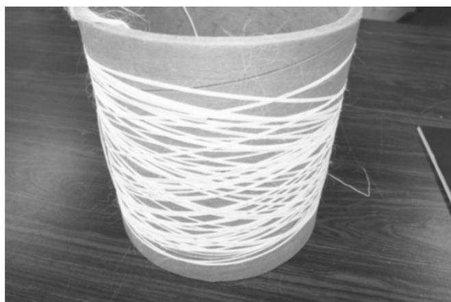
**Figure 3.** A spool of green  $\text{La}_{0.55}\text{Li}_{0.35}\text{TiO}_3$  fiber of  $15\ \mu\text{m}$  diam.
