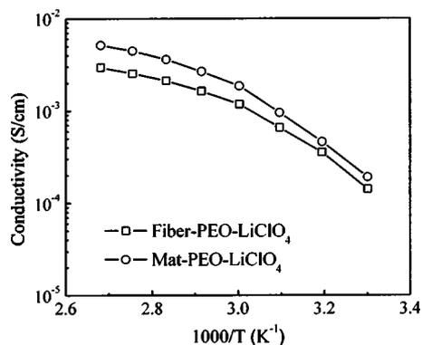
**Figure 10.** Arrhenius plots for ionic conductivities of 50 wt % La<sub>0.55</sub>Li<sub>0.35</sub>TiO<sub>3</sub> fiber-PEO-LiClO<sub>4</sub> and 70 wt % La<sub>0.55</sub>Li<sub>0.35</sub>TiO<sub>3</sub> mat-PEO-LiClO<sub>4</sub> composite electrolytes.
