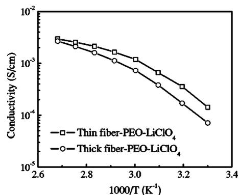
Figure 7. Arrhenius plots for the ionic conductivity of 50 wt %  $\text{La}_{0.55}\text{Li}_{0.35}\text{TiO}_3$  fiber-PEO- $\text{LiClO}_4$  composite electrolytes with differing fiber diameters. Thin fiber: 15  $\mu\text{m}$ , thick fiber: 250  $\mu\text{m}$ .
