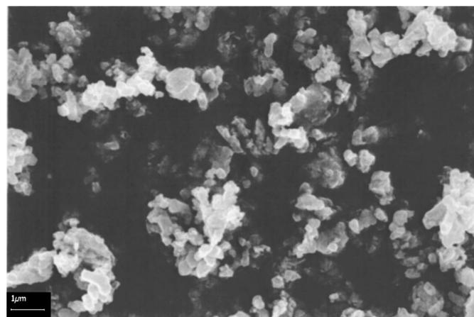
**Figure 2.** SEM images of the  $\text{La}_{0.55}\text{Li}_{0.35}\text{TiO}_3$  particles prepared by solid-state reaction.
