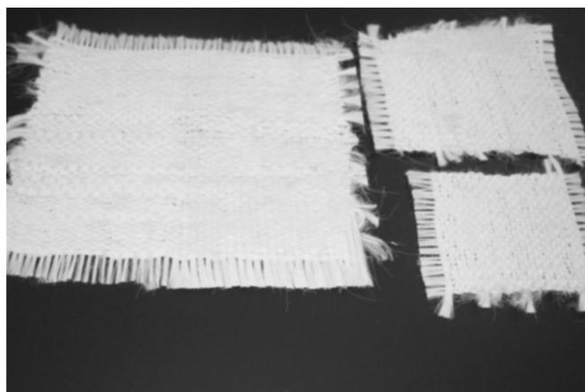
**Figure 4.** Woven mats made from green  $\text{La}_{0.55}\text{Li}_{0.35}\text{TiO}_3$  fibers of  $15\ \mu\text{m}$  diam.
