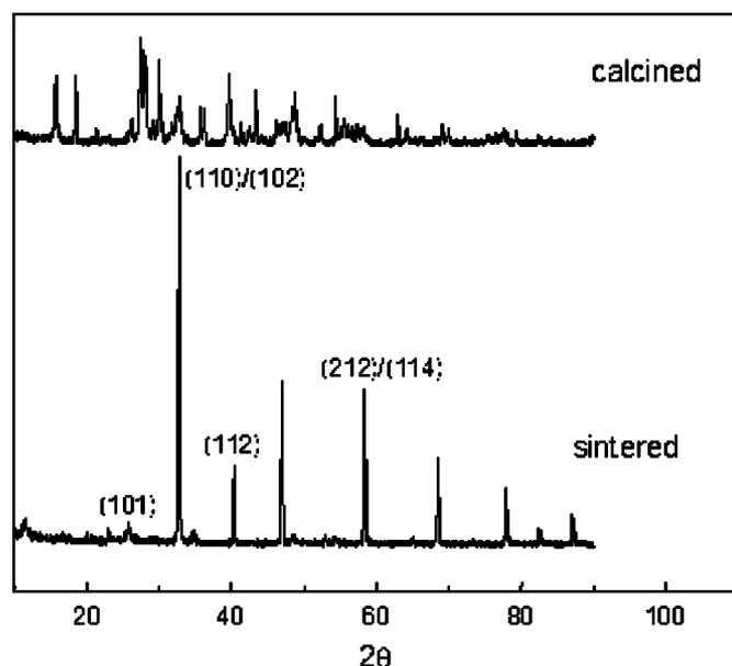
**Figure 1.** XRD patterns of  $\text{La}_{0.55}\text{Li}_{0.35}\text{TiO}_3$  powders calcined at  $800^\circ\text{C}$  and sintered at  $1325^\circ\text{C}$ .
