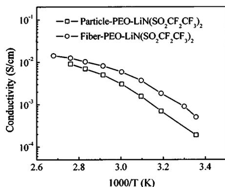
Figure 6. Arrhenius plots for the ionic conductivity of 20 wt %  $\text{La}_{0.55}\text{Li}_{0.35}\text{TiO}_3$  particle-PEO- $\text{LiN}(\text{SO}_2\text{CF}_2\text{CF}_3)_2$  and 20 wt % 250  $\mu\text{m}$  diameter  $\text{La}_{0.55}\text{Li}_{0.35}\text{TiO}_3$  fiber-PEO- $\text{LiN}(\text{SO}_2\text{CF}_2\text{CF}_3)_2$  composite electrolytes.
