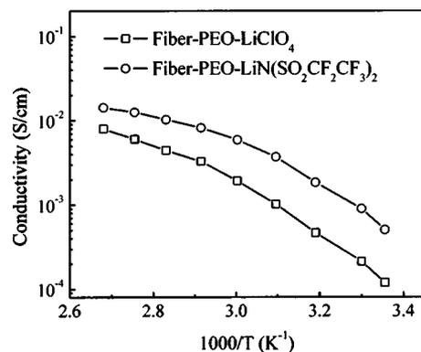
Figure 8. Arrhenius plots for the ionic conductivity of 20 wt %  $\text{La}_{0.55}\text{Li}_{0.35}\text{TiO}_3$  250  $\mu\text{m}$  diam fiber-PEO- $\text{LiClO}_4$  and PEO- $\text{LiN}(\text{SO}_2\text{CF}_2\text{CF}_3)_2$  composite electrolytes.
