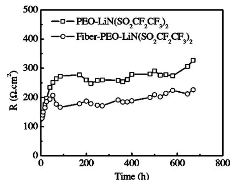
**Figure 11.** Interfacial resistances as a function of time for PEO-LiN(SO<sub>2</sub>CF<sub>2</sub>CF<sub>3</sub>)<sub>2</sub> and 20 wt % 250  $\mu\text{m}$  diam La<sub>0.55</sub>Li<sub>0.35</sub>TiO<sub>3</sub> fiber-PEO-LiN(SO<sub>2</sub>CF<sub>2</sub>CF<sub>3</sub>)<sub>2</sub> polymer electrolytes.
