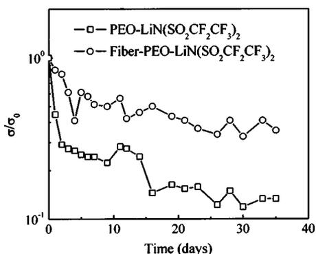
**Figure 9.** Relative conductivity ( $\sigma/\sigma_0$ ) vs. time for PEO-LiN(SO<sub>2</sub>CF<sub>2</sub>CF<sub>3</sub>)<sub>2</sub> and 20 wt % 250  $\mu\text{m}$  diameter La<sub>0.55</sub>Li<sub>0.35</sub>TiO<sub>3</sub> fiber-PEO-LiN(SO<sub>2</sub>CF<sub>2</sub>CF<sub>3</sub>)<sub>2</sub> composite electrolytes.
