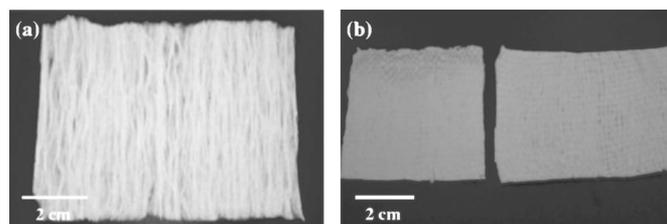
Figure 5. Sintered  $\text{La}_{0.55}\text{Li}_{0.35}\text{TiO}_3$  (a) fibers and (b) mats.
