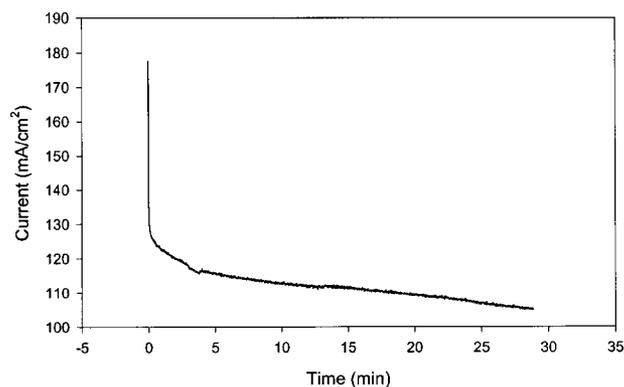
Figure 3. The dependence of current on time of a FC when cell voltage was stepped from open-circuit voltage to 0.4 V. Anode MH with 0.3 wt % Pt as Pt/C, cathode MnO<sub>2</sub>. Catalyst loading 60 mg/cm<sup>2</sup> at both electrodes.
