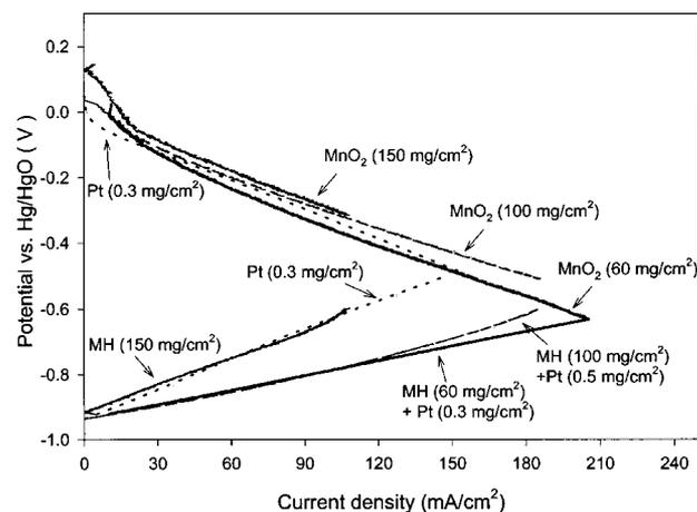
Figure 2. I-E performance of MH (LmNi<sub>4.1</sub>Co<sub>0.4</sub>Mn<sub>0.4</sub>Al<sub>0.3</sub>) anode-MnO<sub>2</sub> cathode AFCs as a function of catalyst loading. The performance of an AFC with commercial Zetek Pt/C electrodes (0.3 mg/cm<sup>2</sup> loading) is also shown for comparison. Performance measured by CV at 1.0 mV s<sup>-1</sup> with H<sub>2</sub> and O<sub>2</sub> as fuel at 25°C.
