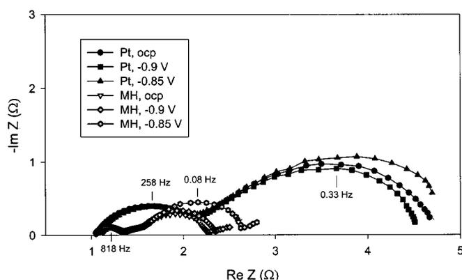
**Figure 8.** Impedance spectra of MH and Pt AFC anodes at different potentials. Frequencies indicated in plots. MH anode loading: 60 mg/cm<sup>2</sup> + 0.3 mg/cm<sup>2</sup> Pt, Pt catalyst loading: 0.3 mg/cm<sup>2</sup>.
