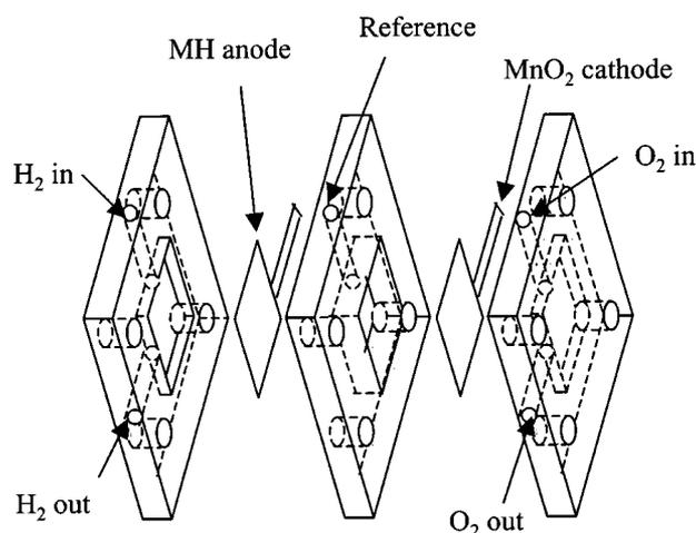
Figure 1. Structure of laboratory MH/MnO<sub>2</sub> AFC.
