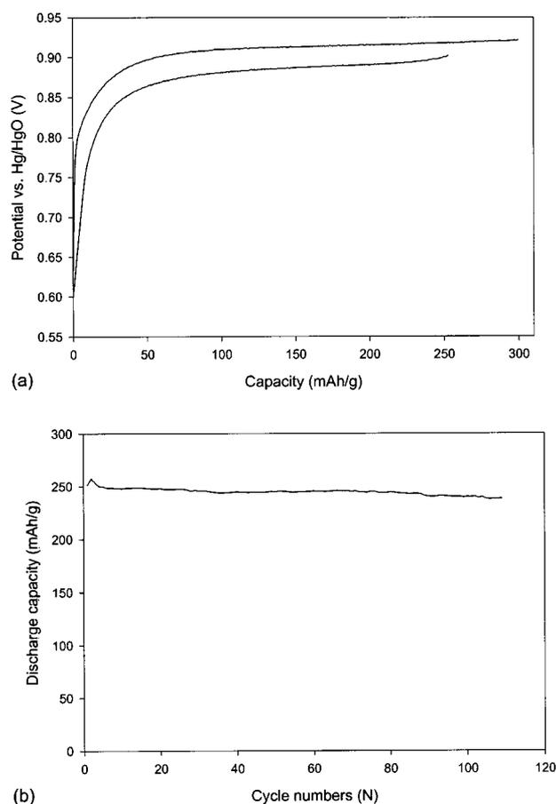
**Figure 6.** (a) The charge/discharge behavior and (b) cycling stability of MH anodes in alkaline electrolytes. The electrode was charged at 50 mA/g for 6.0 h and then discharged at 50 mA/g to  $-0.6$  V vs. Hg/HgO.
