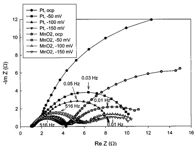
**Figure 9.** Impedance spectra of MnO<sub>2</sub> and Pt AFC cathodes at different potentials. The numbers in the plots indicate the frequency. MnO<sub>2</sub> loading: 60 mg/cm<sup>2</sup>. Pt loading, as Fig. 8.
