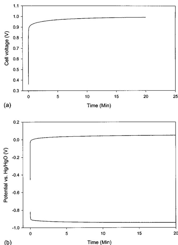
**Figure 5.** The (a) cell voltage and (b) potential changes of MH and MnO<sub>2</sub> anodes and cathodes as a function of recharging via reaction with gaseous H<sub>2</sub> and O<sub>2</sub> after I-E measurement by CV at 1.0 mV/s. MH and MnO<sub>2</sub> loadings 60 mg/cm<sup>2</sup>.
