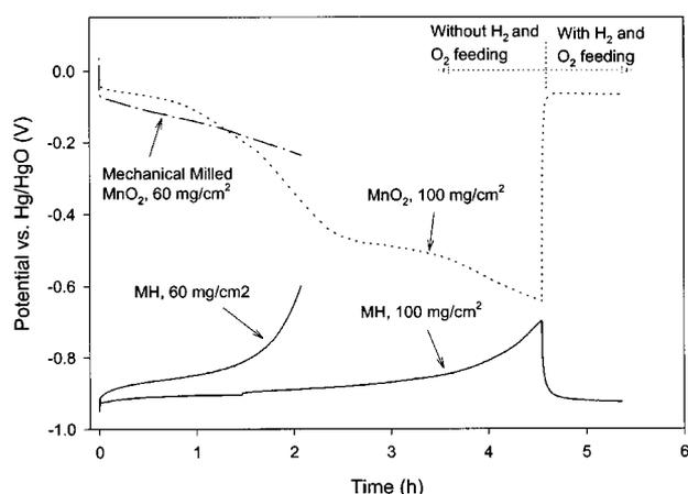
**Figure 4.** The potential behavior of MH/MnO<sub>2</sub> FC at a discharge current of 14 mA/cm<sup>2</sup> after H<sub>2</sub> and O<sub>2</sub> were shut off. For the AFC with 100 mg/cm<sup>2</sup> MH and MnO<sub>2</sub> loadings, H<sub>2</sub> and O<sub>2</sub> were supplied again when the potential of the MnO<sub>2</sub> cathode decreased to -0.7 V vs. Hg/HgO. The MnO<sub>2</sub> cathode with 60 mg/cm<sup>2</sup> loading was mechanically milled for 50 h.
