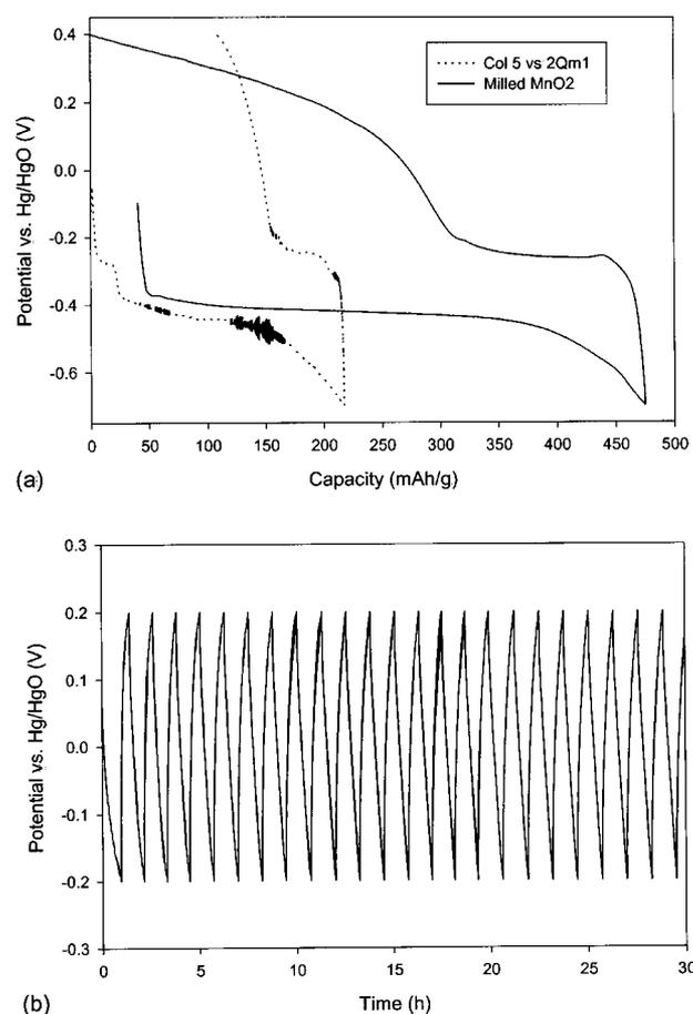
**Figure 7.** (a) The discharge/charge behavior of original and milled  $\text{MnO}_2$  cathode cycling between  $+0.4$  and  $-0.7$  V in 6 M KOH electrolytes, and (b) cycling stability of milled  $\text{MnO}_2$  cathode cycling between  $+0.2$  and  $-0.2$  V. Cycling current: 50 mA/g.
