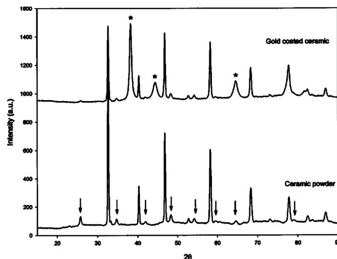
**Figure 3.** XRD patterns of  $\text{La}_{0.55}\text{Li}_{0.35}\text{TiO}_3$  powder and Au-coated  $\text{La}_{0.55}\text{Li}_{0.35}\text{TiO}_3$  sheet. Arrows denote superstructure peaks of the perovskite, and (\*) the Au line.
