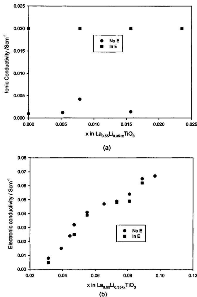
**Figure 10.** (a) Ionic and (b) electronic conductivities of a sintered La<sub>0.55</sub>Li<sub>0.35</sub>TiO<sub>3</sub> disk electrode as a function of Li intercalation levels using GITT.
