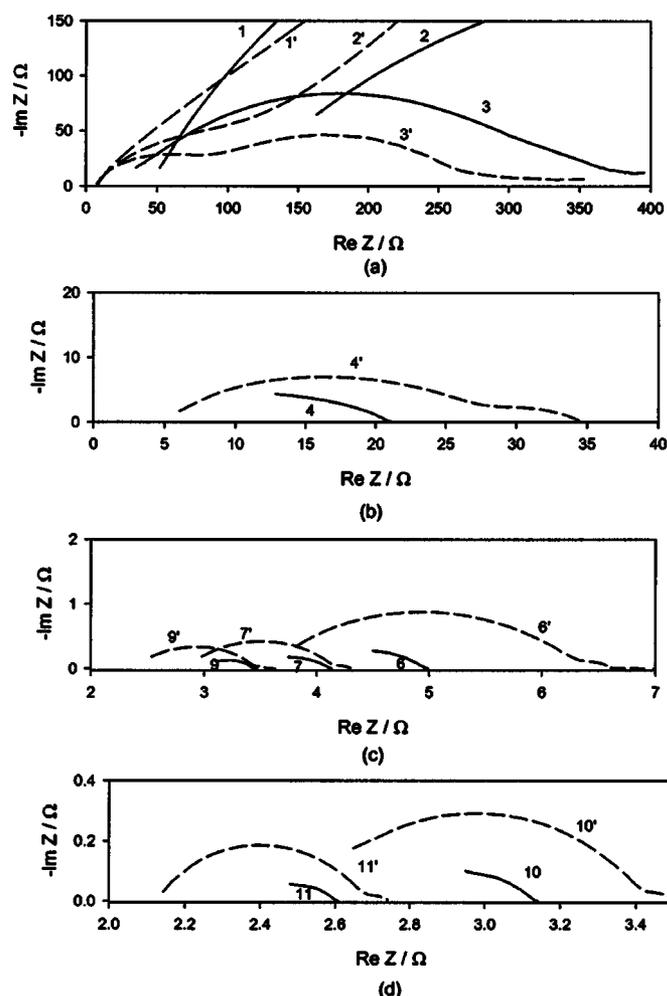
**Figure 11.** Impedance of the sintered La<sub>0.55</sub>Li<sub>0.35</sub>TiO<sub>3</sub> disk electrode in Fig. 8 with and without interference by liquid electrolyte: (—) without electrolytes and (---) immersed in electrolyte.
