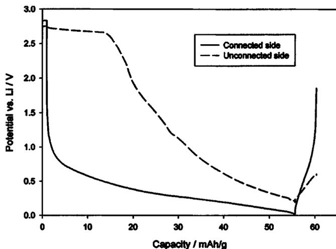
**Figure 4.** Potentials at the charge-discharge side and the unconnected side of  $\text{Li}_{0.55}\text{La}_{0.35}\text{TiO}_3$  on the first Li insertion-extraction at 1.0 mA/g current.
