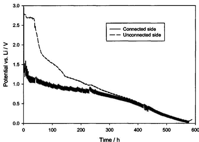
**Figure 5.** Potentials at the charging side and unconnected side as a function of time for the first Li insertion cycle in  $\text{La}_{0.55}\text{Li}_{0.35}\text{TiO}_3$  using GITT. Charge current 0.5 mA/g. The intermittent current was applied for 2.0 h, then switched off for 2.0 h.
