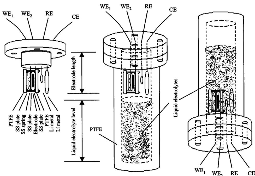
**Figure 1.** PTFE cell configuration designed for *in situ* electrical conductivity measurement of sintered  $\text{La}_{0.55}\text{Li}_{0.35}\text{TiO}_3$  disk electrode at different Li insertion levels without influence of liquid electrolytes. The ceramic electrode was charged-discharged in an inverted position, and then the electric conductivity was measured at the same Li insertion levels by EIS with the cell in an upright position.
