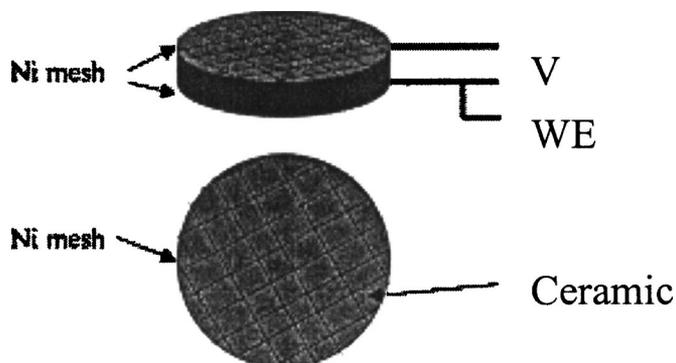
**Figure 2.** Schematic diagram of ceramic powder electrode configuration.
