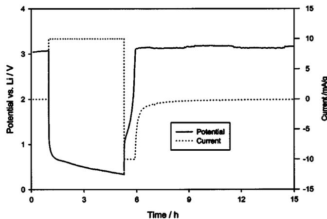
**Figure 6.** The dependence of the potential and current of  $\text{La}_{0.55}\text{Li}_{0.35}\text{TiO}_3$  powder electrode during charge (Li insertion) and discharge (Li extraction) in a liquid electrolyte between 0.33 and 4.2 V. Before charge/discharge, the electrode was at open circuit for 1 h.
