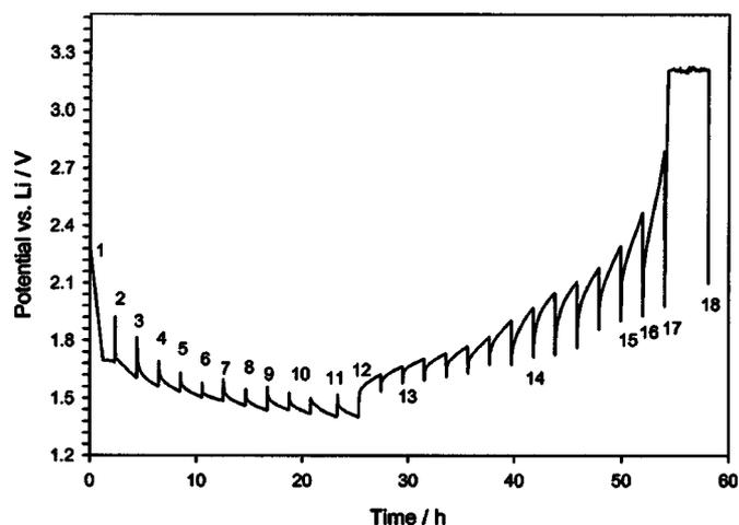
**Figure 8.** Charge-discharge profiles of a sintered  $\text{La}_{0.55}\text{Li}_{0.35}\text{TiO}_3$  disk electrode as a function of charge/discharge time using GITT. The charge current of 0.6 mA/g and discharge current of 0.5 mA/g were switched on for 2.0 h and off for 2.0 h before EIS measurement.
