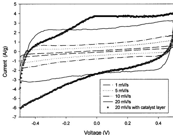
**Figure 4.** CV of  $\text{RuO}_2 \cdot x\text{H}_2\text{O}$  supercapacitor at different scan rates.  $\text{RuO}_2 \cdot x\text{H}_2\text{O}$  loading 1.0 mg  $\text{cm}^{-2}$  with 30 wt % Nafion for both anodic and cathodic sublayers.
