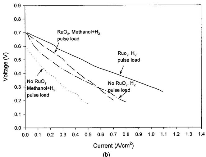
**Figure 11.** Voltage for methanol/hydrogen cell vs. current density with supercapacitive sublayers on both anode and cathode sides (loading as Fig. 9). The methanol was fed by passing hydrogen through 50 vol % water/methanol mixture at  $50^\circ\text{C}$ . Anode electrocatalyst ( $\text{Pt}_1\text{Ru}_1$ ) loading  $0.6 \text{ mg cm}^{-2}$ , Pt cathode loading as Fig. 6,  $\text{RuO}_2 \cdot x\text{H}_2\text{O}$  sublayer loadings as Fig. 9. Nafion 112 membrane.
