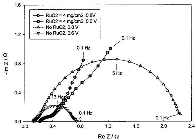
**Figure 7.** Impedances of hydrogen/air PEMFC with and without  $4.0 \text{ mg cm}^{-2}$   $\text{RuO}_2 \cdot x\text{H}_2\text{O}$  sublayers at 0.8 and 0.6 V cell voltages. Cell performances shown in Fig. 6. Electrocatalyst loadings as in Fig. 6.
