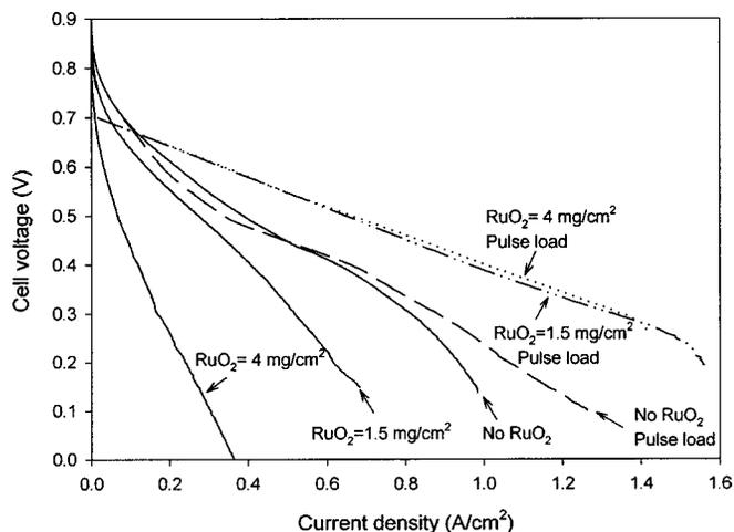
**Figure 6.** Performance of hydrogen/air PEMFC with different  $\text{RuO}_2 \cdot x\text{H}_2\text{O}$  loadings at steady-state and pulsed loads. Steady-state performance measured by CV at  $1.0 \text{ mV s}^{-1}$ ; pulse-load performance measured by the pulse voltammetry program in Fig. 3. Platinum anode and cathode electrocatalyst loading  $0.17 \text{ mg cm}^{-2}$ . Nafion 112 membrane.
