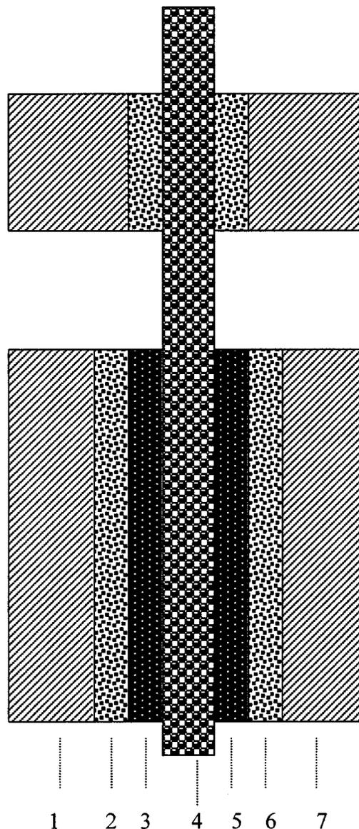
**Figure 2.** Schematic structure of a multilayer electrode MEA: (1) anode GDL; (2) anode electrocatalyst layer; (3) supercapacitive sublayer; (4) Nafion membrane; (5) supercapacitive sublayers; (6) cathode electrocatalyst layer; and (7) cathode GDL.
