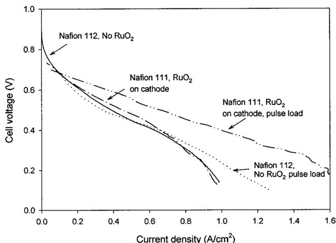
**Figure 10.** Performance of hydrogen/air PEMFC with SL on cathode side (loadings as Fig. 9) with Nafion 111 electrolyte. The cell with Nafion 112 without supercapacitive sublayers is shown for comparison.
