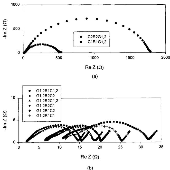
**Figure 3.** Impedances of two CEs ( $C_1$  and  $C_2$ ) and (b) graphite electrode ( $G_{1,2}$ ) in five-electrode cell with configuration of  $C_2(\text{Li})-R_2(\text{Li})-G_{1,2}-R_1(\text{Li})-C_1(\text{Li})$ . The EIS was measured after relaxation for 2.0 h after the third discharge to 0.0 V.  $C_{1,2}$ : Indicating  $C_1$  and  $C_2$  are connected together as CEs.  $G_{1,2}$ : As Fig. 2.
