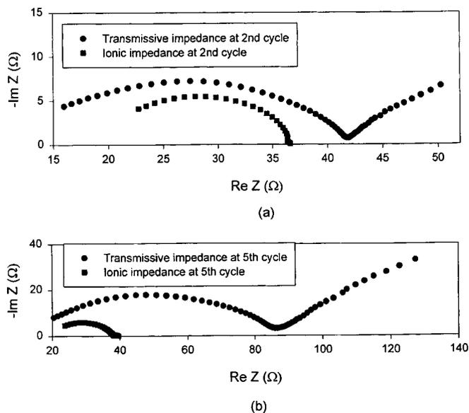
**Figure 7.** Transmissive and ionic impedances of  $\text{Sn}_{1.3}\text{Al}_{0.3}\text{Ti}_{2.3}\text{O}_{1.95}(\text{PO}_4)_3$  measured after 5.0 h relaxation following the 2nd and 6th discharge to 0.0 V. The transmissive impedance was measured by connecting  $RE_2$  and WE terminal of the Solatron interface together to  $T_1$  side, and  $RE_1$  plus CE to  $T_2$  side. The ionic impedance was measured by using four-probe measurement.
