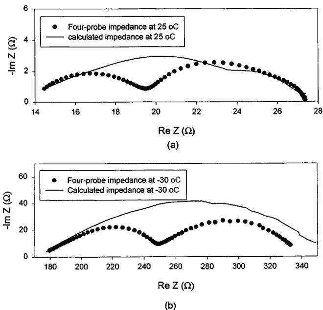
**Figure 5.** Impedances of electrolytes between REs  $R_1$  and  $R_2$  using four-probe measurement after 3rd discharge to 0.0 V at 25°C and after 6th discharge to 0.0 V at -30°C. Electrolyte impedances calculated from Eq.  $Z_{\text{ion}} = Z_{G_3C_2} - Z_{G_3R_1G_{1,2}} - Z_{C_2R_2G_{1,2}}$  also shown in Fig. 4 to check validity of electrolyte impedance using four-probe method.
