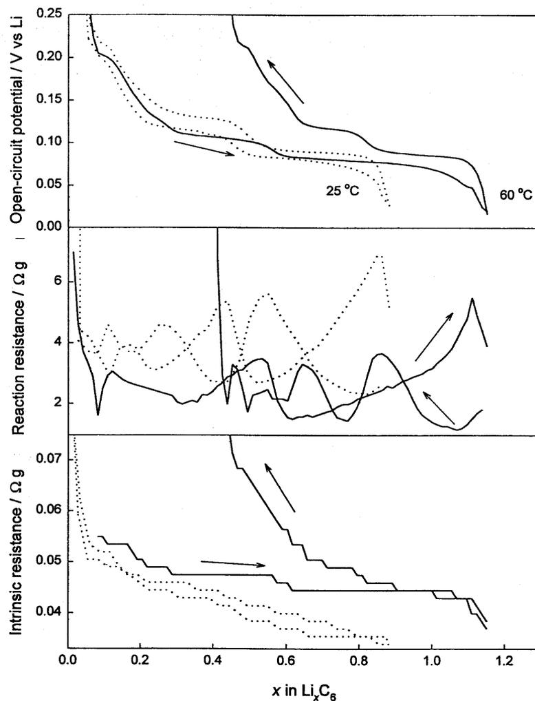
Fig. 12. Open-circuit potential, intrinsic resistance and reaction resistance for JM 287 electrode at 25 and 65°C. 25°C data measured after 17 cycles, 65°C data after 3 cycles, both at the experimental temperature. Charge–discharge current: 5.1 mA g<sup>-1</sup>. Galvanostatic current pulses were on for 1.0 h, off for 2.5 h.
