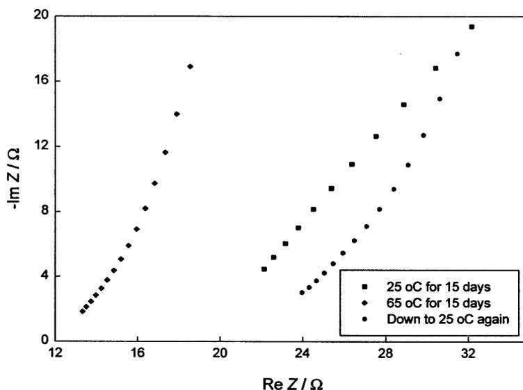
Fig. 11. High frequency spectra Nyquist plots for palladium wire electrode in the experimental electrolyte at 25 and 65°C.
