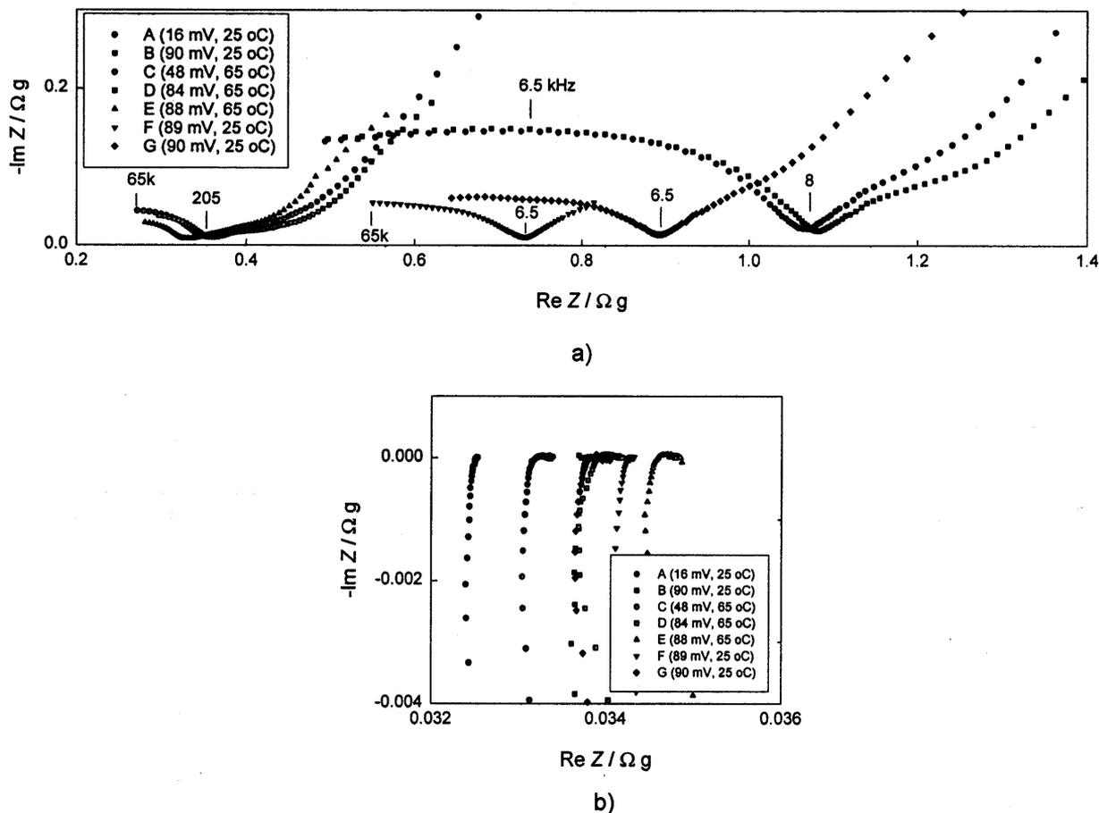
Fig. 9. Nyquist plots for JM 287 electrode at 25 and 65°C (points A–G, Fig. 8). (a) For lithium insertion–extraction kinetics measured using C protocol; (b) Intrinsic resistance measured using A protocol.
