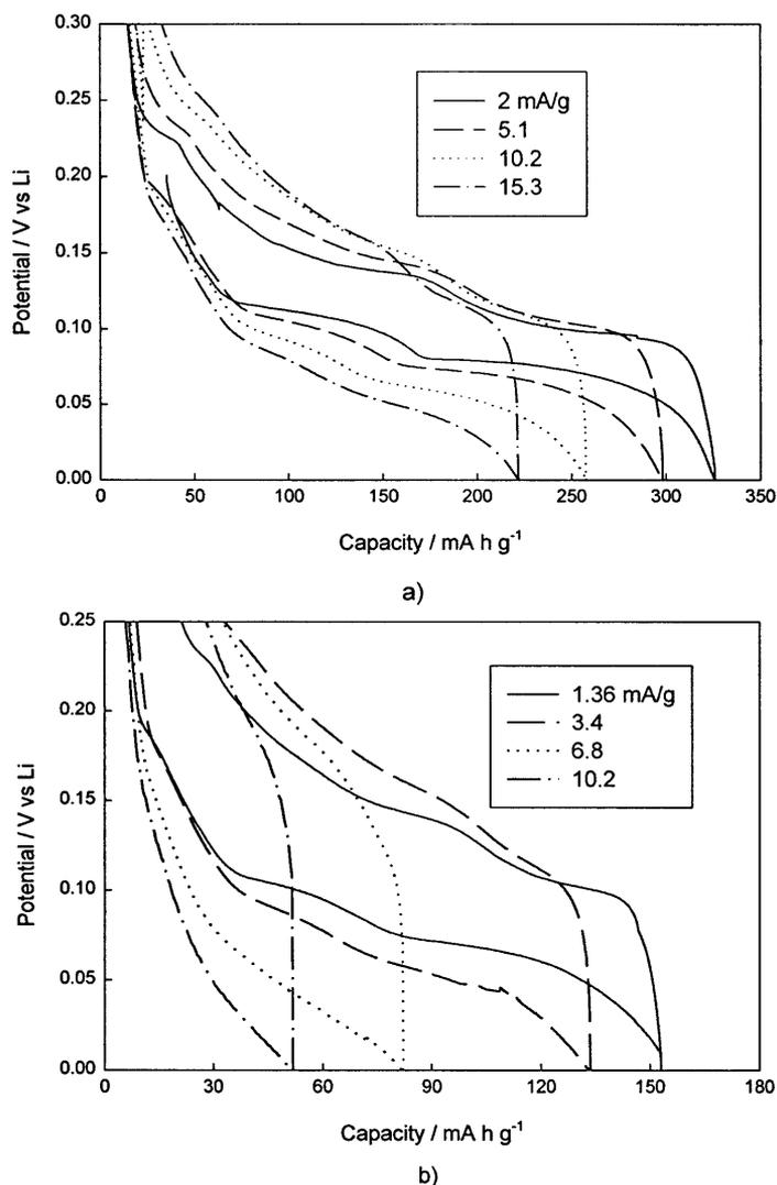
Fig. 2. Potential profiles as a function of cycle current after 9 previous cycles. (a) JM 287; (b) MCMB 10-28.
