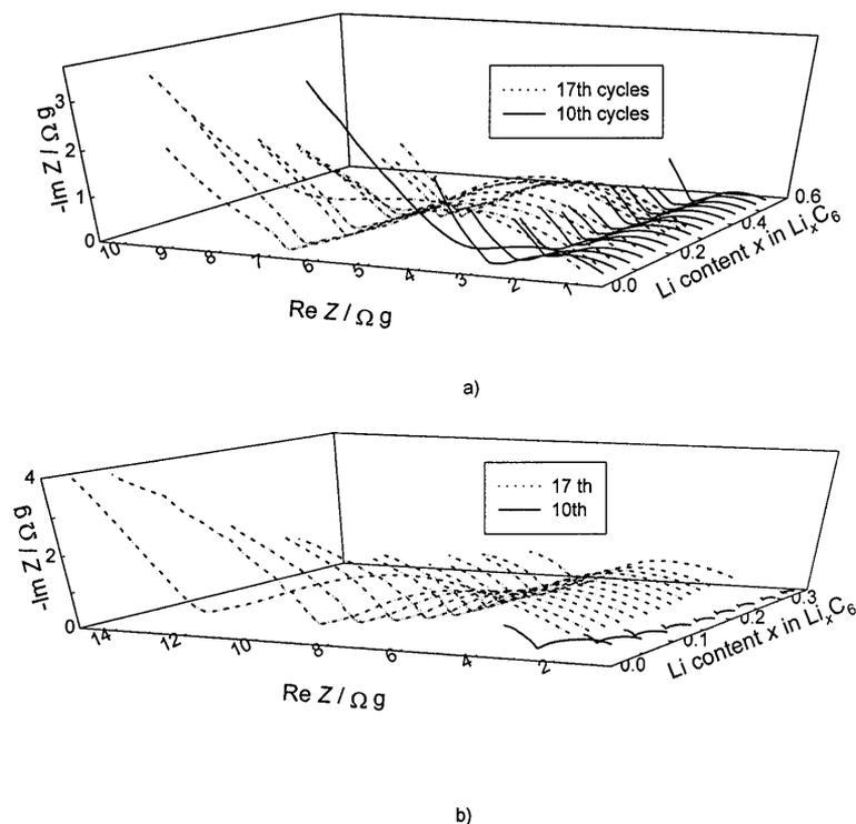
Fig. 4. Nyquist plots demonstrating: (a) kinetics of lithium insertion–extraction; (b) intrinsic impedance of MCMB 10-28 graphite as a function of lithium content on cycles 10 and 17.
