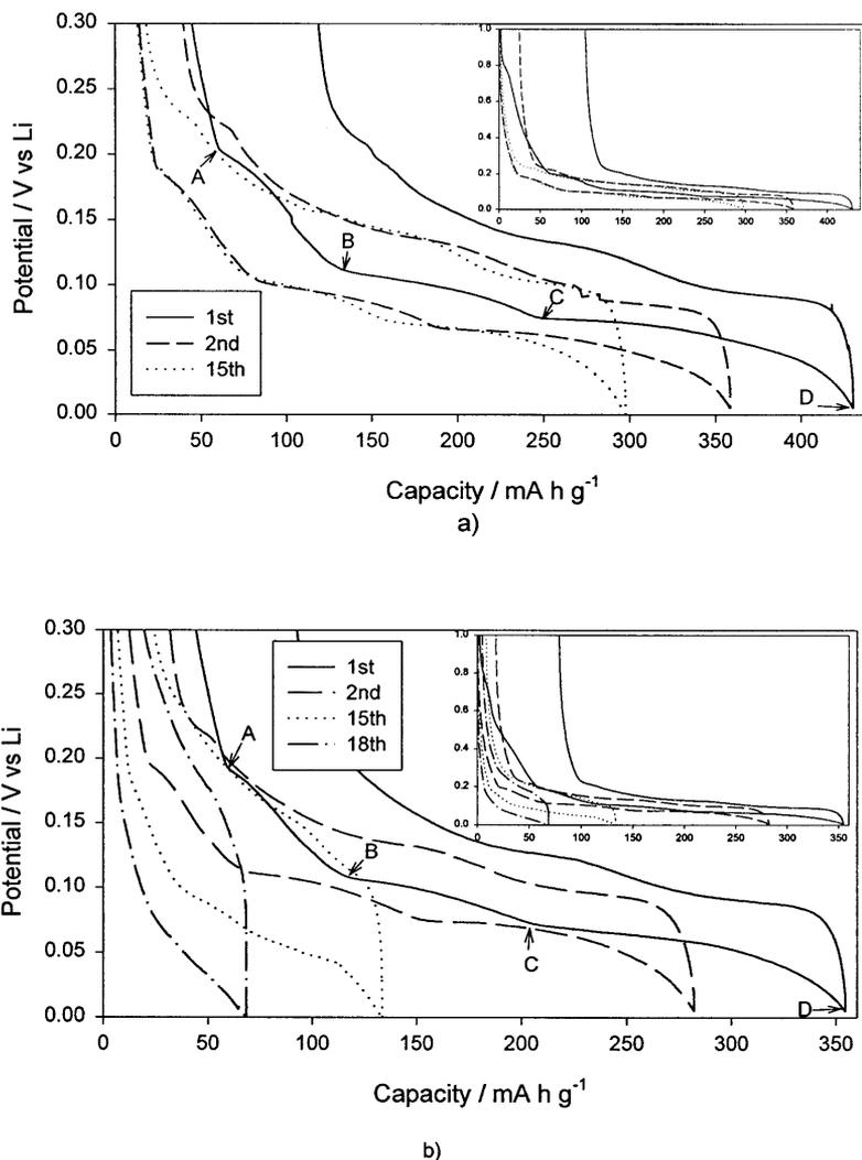
Fig. 1. Potential profiles of graphite electrodes during charge–discharge cycles 1, 2, and 15. A–B, B–C, and C–D correspond to the lithium capacity of the three phase zones. (a) JM 287; cycling current,  $5.1 \text{ mA g}^{-1}$ ; (b) MCMB 10-28; cycling current,  $3.4 \text{ mA g}^{-1}$ . The insets in the right corner show the expanded potential range.
