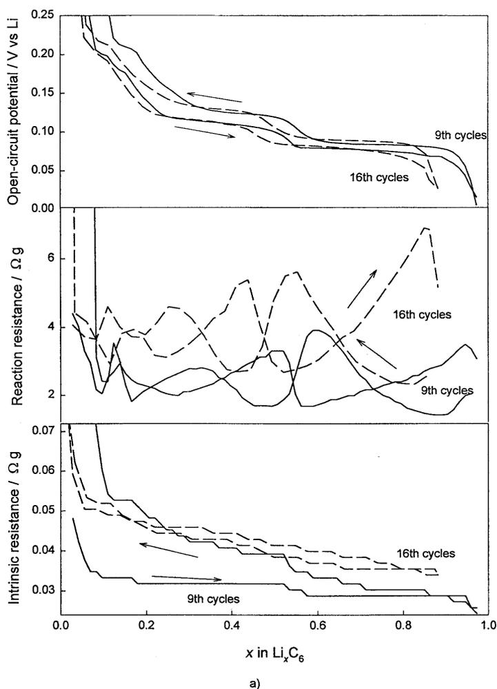
Fig. 3. Dependence of open-circuit potential, intrinsic resistance and reaction resistance on cycles 9 and 16. Charge–discharge current: 5.1 mA g<sup>-1</sup>. Galvanostatic current pulses are on for 1.0 h, off for 2.5 h. (a) JM 287; (b) MCMB 10-28.
