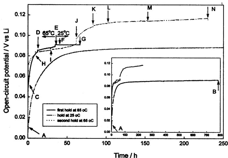
Fig. 8. Potential profiles of JM 287 electrode on open circuit at 25 and 65°C as a function of time. The fully charged JM 287 graphite electrode was first left on open-circuit at 25°C for 800 h (point A–B), then was again fully charged, left at 65°C for 35 h, then again left at 25°C for 32 h (point C–G). After 3 charge–discharge cycles at 65°C the fully charged JM 287 graphite was held at 65°C for 230 h (point H–N). EIS results were obtained at A–N.
