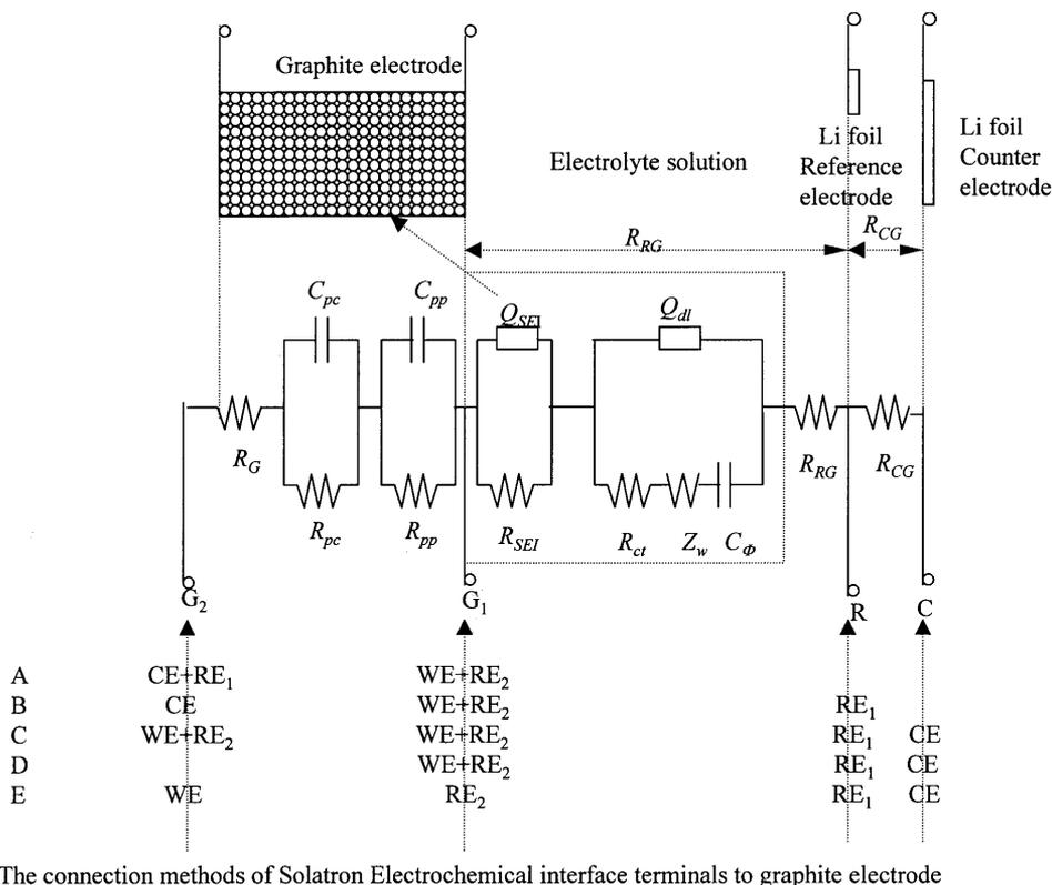
Fig. 6. Equivalent circuit of graphite electrodes (modified from Funabiki Ref. [7]). A schematic diagram of the cell and different Solatron electrochemical interface terminal-to-electrode connections (Fig. 7) is also shown.
