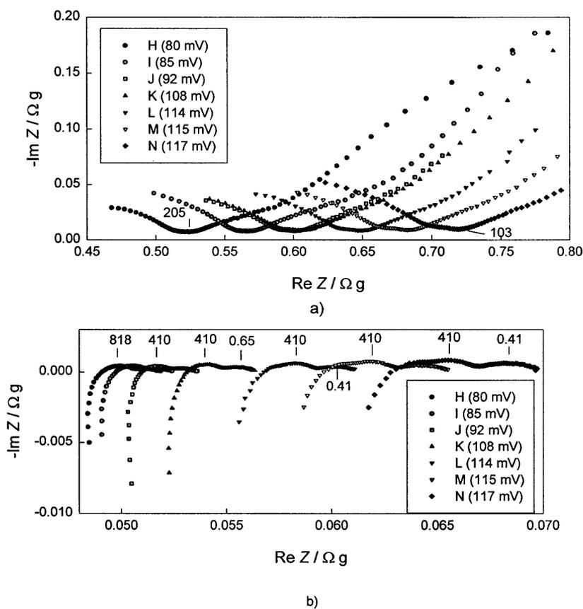
Fig. 10. Nyquist plots for JM 287 electrode at 65°C (point H–N, Fig. 8). (a) For lithium insertion–extraction kinetics measured using C protocol; (b) Intrinsic resistance measured using A protocol.
