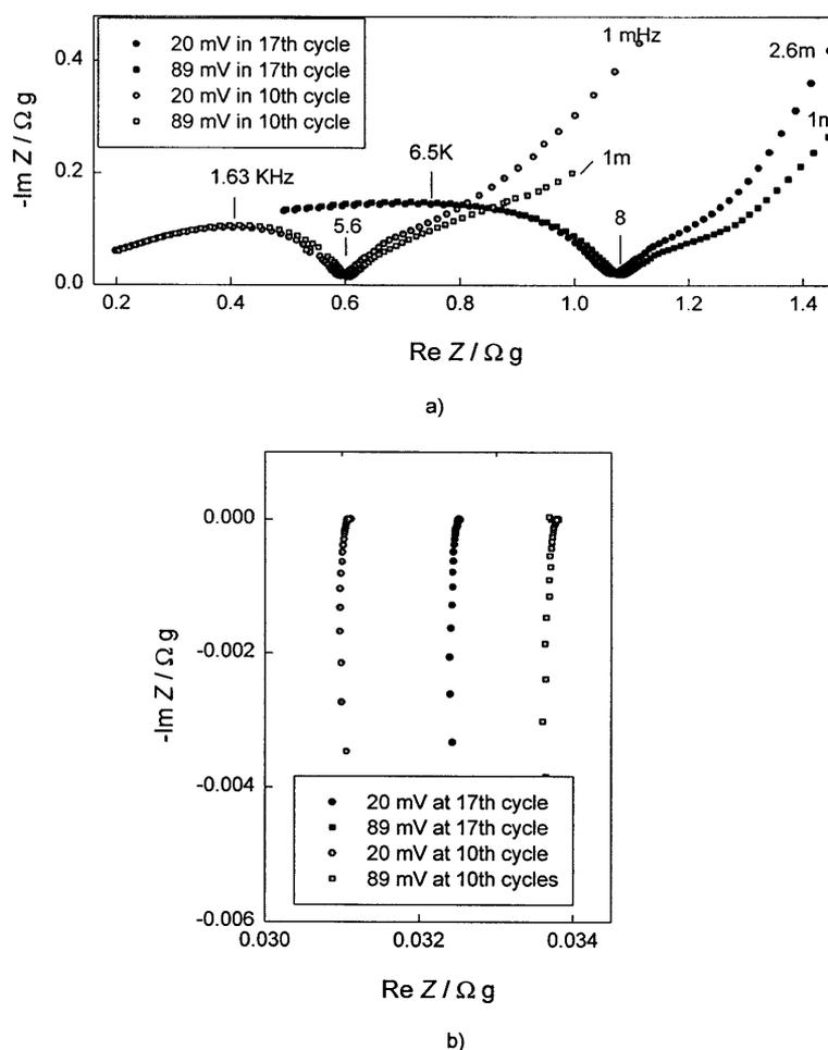
Fig. 5. Nyquist plots demonstrating: (a) kinetics of lithium insertion–extraction; (b) intrinsic impedance of JM 287 graphite at potentials of 20 and 89 mV, cycles 10 and 17.
