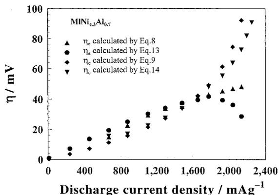
Fig. 5. Electrochemical overpotential  $\eta_e$  and concentration overpotential  $\eta_c$  in  $\text{MINi}_{4.3}\text{Al}_{0.7}$  hydride electrodes calculated by different expressions.
