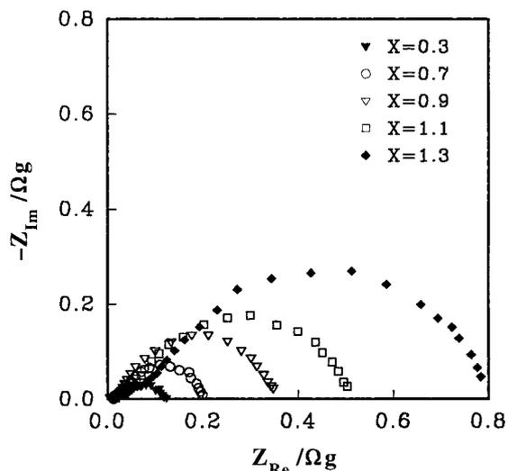
Fig. 3. Electrochemical impedance spectra of the  $\text{MINi}_{4.3-x}\text{Co}_x\text{Al}_{0.7}$  electrodes at  $X=0.3, 0.7, 0.9, 1.1$  and  $1.3$ .
