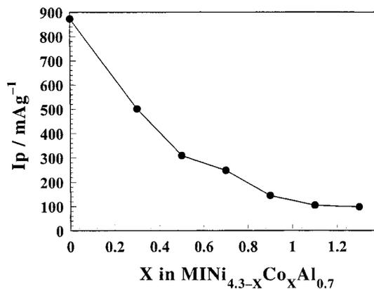
Fig. 11. Peak current density  $I_p$  dependence of Co content in  $\text{MINi}_{4.3-x}\text{Co}_x\text{Al}_{0.7}$  hydride electrodes.
