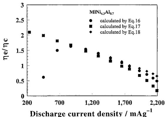
Fig. 8. The ratio of electrochemical overpotential  $\eta_e$  to concentration overpotential  $\eta_c$  in  $\text{MINi}_{4.3}\text{Al}_{0.7}$  hydride electrodes calculated by different expressions.
