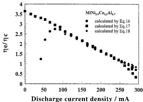
Fig. 10. The ratio of electrochemical overpotential  $\eta_e$  to concentration overpotential  $\eta_c$  in  $\text{MINi}_{3.0}\text{Co}_{1.3}\text{Al}_{0.7}$  hydride electrodes calculated by different expressions.
