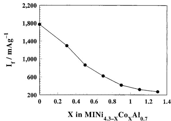
Fig. 13. Critical point current density  $I_f$  dependence of Co content in  $\text{MINi}_{4.3-X}\text{Co}_X\text{Al}_{0.7}$  hydride electrodes.
