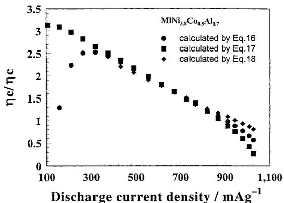
Fig. 9. The ratio of electrochemical overpotential  $\eta_e$  to concentration overpotential  $\eta_c$  in  $\text{MINi}_{3.8}\text{Co}_{0.5}\text{Al}_{0.7}$  hydride electrodes calculated by different expressions.
