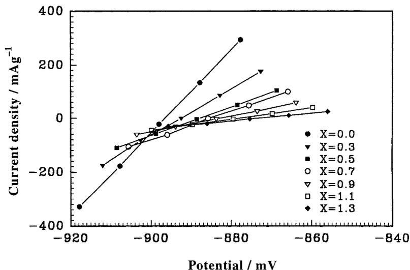
Fig. 2. Linear polarization curves of  $\text{MINi}_{4.3-x}\text{Co}_x\text{Al}_{0.7}$  hydride electrodes.
