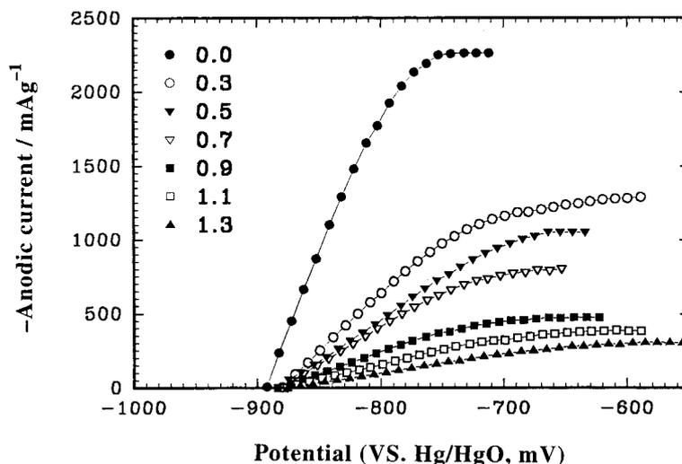
Fig. 4. Anodic polarization of  $\text{MINi}_{4.3-x}\text{Co}_x\text{Al}_{0.7}$  hydride electrodes.
