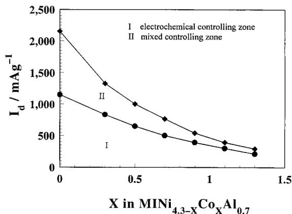
Fig. 14. The electrochemical controlling zone and mixed controlling zone dependence of Co content in  $\text{MINi}_{4.3-X}\text{Co}_X\text{Al}_{0.7}$  hydride electrodes.
