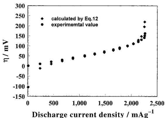
Fig. 12. Comparison of the experimental  $\eta$  (circle) with that calculated by Eq. 15 (rhomb) in  $\text{MINi}_{4.3}\text{Al}_{0.7}$  hydride electrodes.
