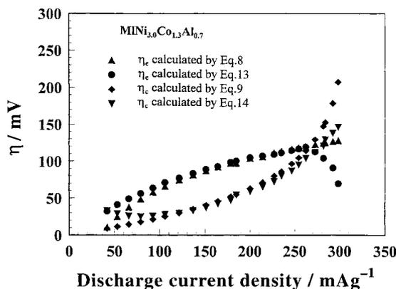
Fig. 7. Electrochemical overpotential  $\eta_e$  and concentration overpotential  $\eta_c$  in  $\text{MINi}_{3.0}\text{Co}_{1.3}\text{Al}_{0.7}$  hydride electrodes calculated by different expressions.
