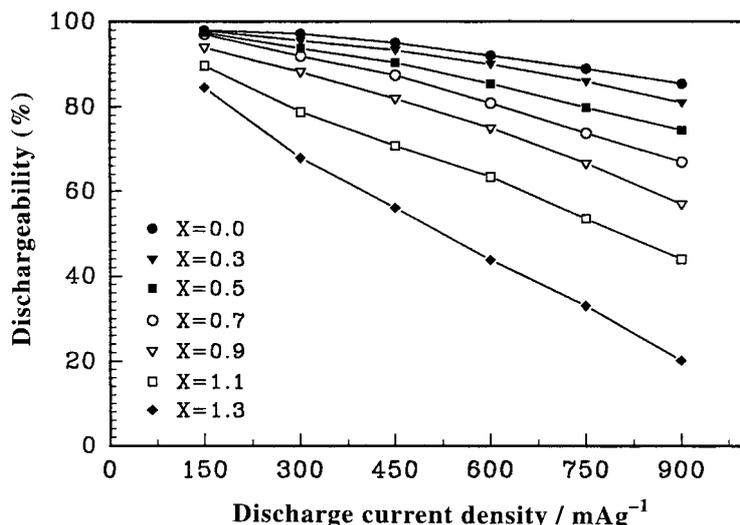
Fig. 1. High rate dischargeability HRD of  $\text{MINi}_{4.3-x}\text{Co}_x\text{Al}_{0.7}$  hydride electrodes.
