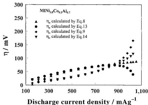
Fig. 6. Electrochemical overpotential  $\eta_e$  and concentration overpotential  $\eta_c$  in  $\text{MINi}_{3.8}\text{Co}_{0.5}\text{Al}_{0.7}$  hydride electrodes calculated by different expressions.
