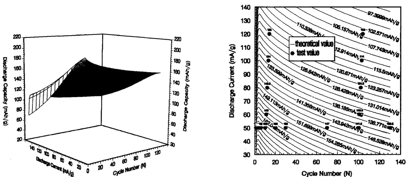
Fig. 2. Plot of the measured values of the capacity for TiNi samples (blank point) and model curve: (a) three-dimensional curved surface; (b) isodischarge capacity section.
