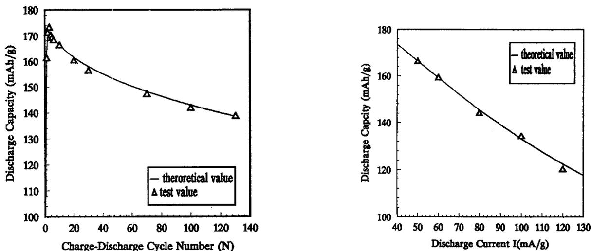
Fig. 3. Plot of model curve vs. measured sample value: (a)  $I = 50 \text{ mA g}^{-1}$ ; (b)  $N = 10$ .
