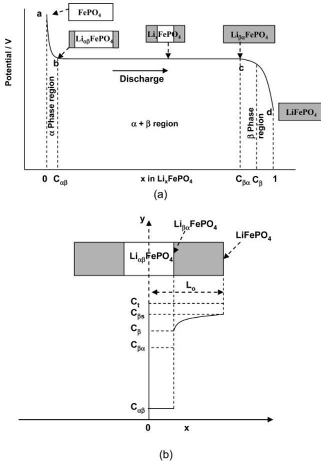
**Figure 1.** Schematic diagram showing (a) phase transformation and (b) Li concentration distribution during the discharge of a  $\text{LiFePO}_4$  particle (Li insertion into  $\text{FePO}_4$ ).
